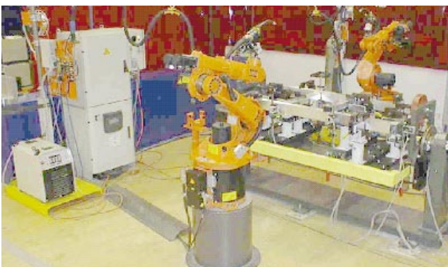
Figure 4. Principal test set-up for symmetrical welding of generic frames.
