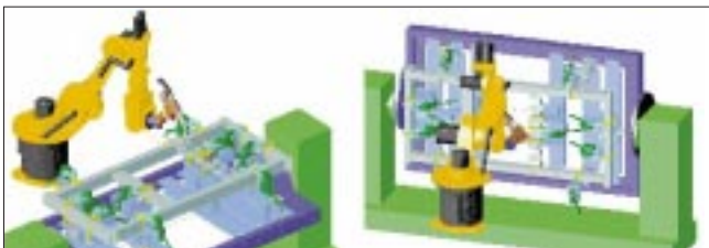
Figure 2. Simulation results from welding access control in different welding positions.
