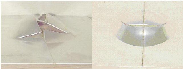
Figure 11. Cracking behaviour of welded aluminium blanks.
