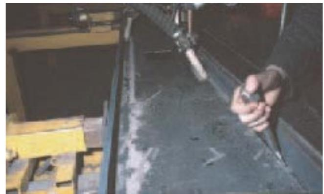
Figure 3. The self-released slag is easily removed.
