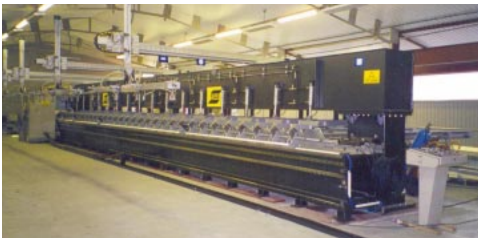
Figure 6. Plant for the friction stir welding of panels from extrusions at Marine Aluminium in Norway.
