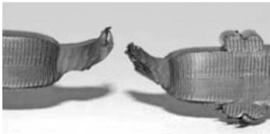
(b) Ductile Rupture Outside Fusion Interface
