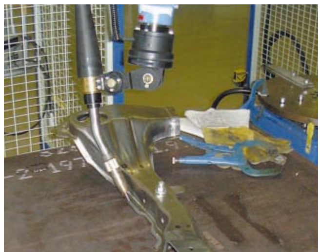
Interior from the robot cell in Göteborg where a front suspension part is test welded with OK Tubrod 14.11 Ø 1.4 mm.
